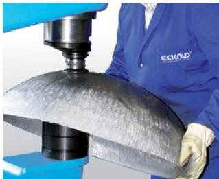
*ECKOLD technology means precise and chipless cold forming of sheet metal and profiles with minimum noise. The same machine is used for bending profiles and forming sheet metal, for making new parts as well as for repairs and the precise correcting of parts. Available for the machines are a wide range of tools which can be mounted and changed in a matter of seconds to suit the work in hand with the machine. This intelligent ECKOLD technology is unique throughout the world.*
