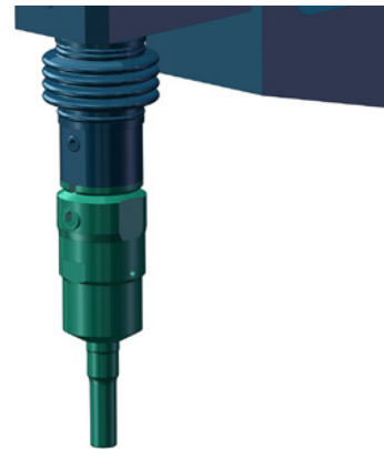
Clinchvariante R-DF, rundes Clinchelement Clinching variant R-DF, round clinching element
