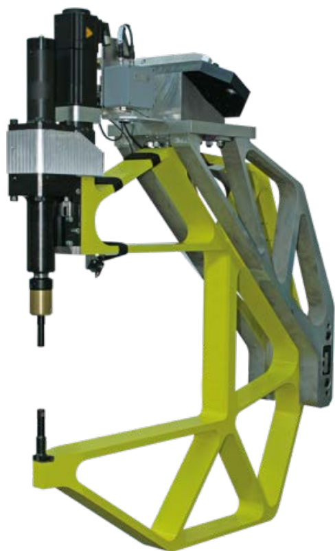
Special clinching frame (weight-optimised)
