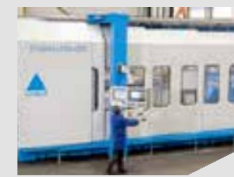
World's strongest flow-forming machine for tube wall thicknesses of up to 50 \text{ mm} (stainless steel)
