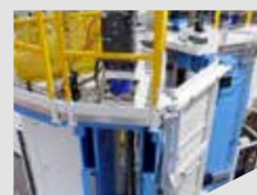
First flow-forming machine for precision tubes with \text{\O} up to 750 \text{ mm} and length of over 5.200 \text{ mm}
