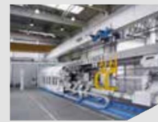
World's largest flow-forming machine for precision tubes up to 13,500 \text{ mm}
