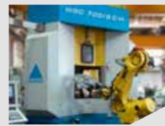
Development of the WSC series for the vertical production of aluminium and steel wheels
