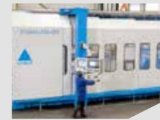
World's strongest flow-forming machine for tube wall thicknesses of up to 50 mm (stainless steel)
