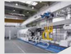
World's largest flow-forming machine for precision tubes up to 13,500 mm
