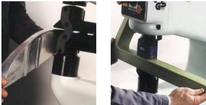
Mostly used for straightening and correcting parts, e.g. when working on aircraft parts.
