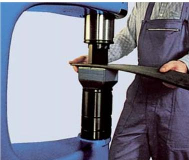
*Parts which have been distorted by welding can be corrected and readjusted by shrinking and stretching with the ECKOLD Kraftformer.*
